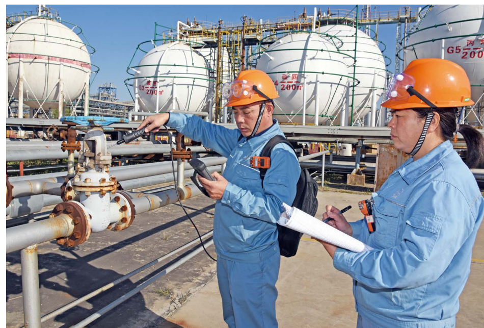
④ Cangzhou Refinery staff conducts VOCs inspections
